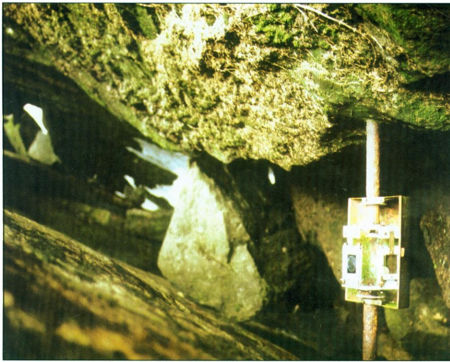
Phot. 8. Piekietko. A view of the crack gauge installed into a fissure of the block field (phot. B. Košťák)
